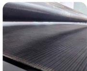
Full-Area Adsorption Platform
