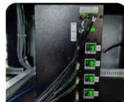
Ink Path Negative Pressure System
